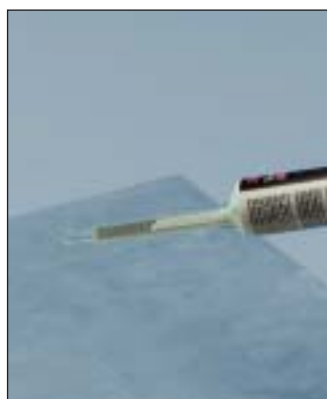
Pull the trigger for exact dispensing, while the adhesives are mixed and applied at once
