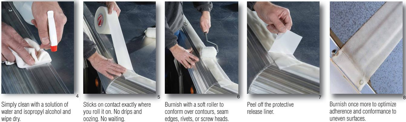
4 Simply clean with a solution of water and isopropyl alcohol and wipe dry.
